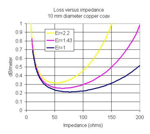
So why 75 ohms? Here's our guess. Often the center conductor of cheap cables is made of a steel core, with some copper plating. The lower the impedance, the bigger the diameter of the center core. An impedance 75 ohms probably was a compromise between low loss and cable flexibility.
