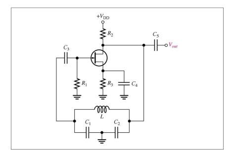
• The Colpitts oscillator utilizes a tank circuit (LC) in the feedback loop. The resonant frequency can be determined by the formula below. Since the input impedance affects the Q, an FET is a better choice for the active device.
