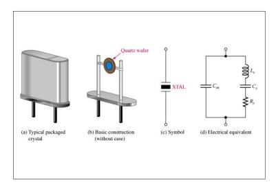
The inductor L and the capacitor C represent electrical equivalents of Crystal mass
