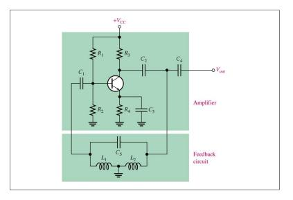
The Hartley oscillator is similar to the Colpitts. The tank circuit has two inductors and one capacitor. The calculation of the resonant frequency is the same.
