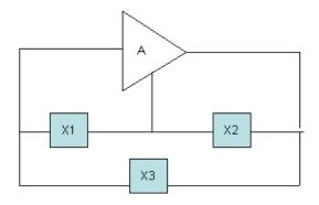
• A variety of circuits can be built using the above diagram, by providing tuning in both the input and output sections of the circuit.
