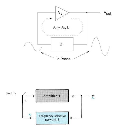
When the switch at the amplifier input is open, there are no oscillations. Imagine that a voltage Vi is fed to the circuit and the switch is closed. This results in Vo = AV Vi and  $\beta$ Vo = Vf is fed back to the circuit. If we make Vf = Vi, then even if we remove the input
