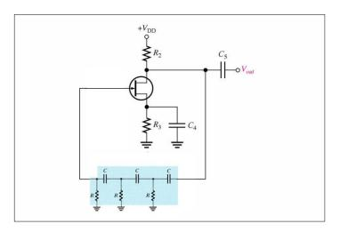
• The amplifier stage is self biased with a capacitor bypassed source resistor Rs and a drain bias resistor RD . The FET device parameters of interest are gm and rd.
