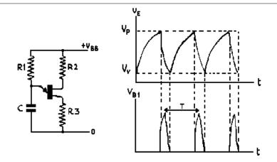
The emitter current then rises rapidly, discharging C1 through the base 1 region and R3. The sudden rise of current through R3 produces the voltage pulse. When the current falls to IV the UJT switches off and the cycle is repeated. Oscillator operating frequency fo =  $1/{\text{RTCTln}[1/(1-\eta)]}$  where,  $\eta$  is
