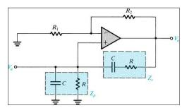
• R and C are used for frequency adjustment and resistors R1 and R2 form part of the feedback path.
