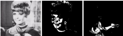
FIGURE 10.39 (a) Original color image shown as a monochrome picture. (b) Segmentation of pixels with colors close to facial tones. (c) Segmentation of red components.
