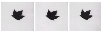
FIGURE 10.43 (a) Original image. (b) Result of split and merge procedure. (c) Result of thresholding (a).
