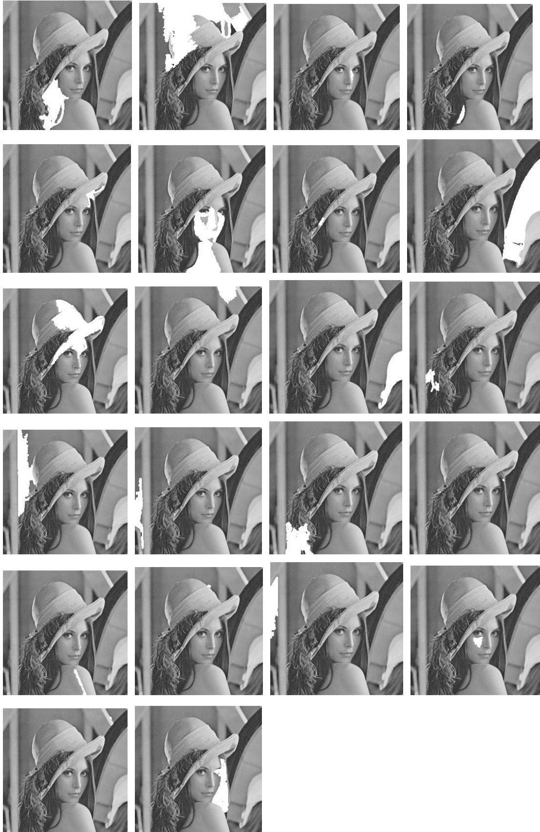
Figure 3.2 Lena image after using region growing, there are 90% pixels have been classified. Threshold/second: 20/4.7 seconds.
