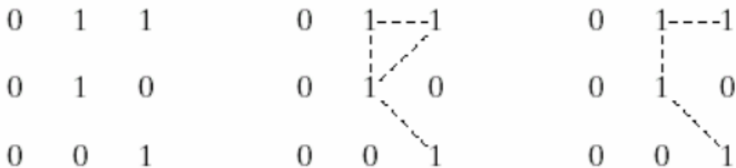
Fig: (a) Arrangement of pixels; (b) pixels that are 8-adjacent to the center pixel (c) m-adjacency
