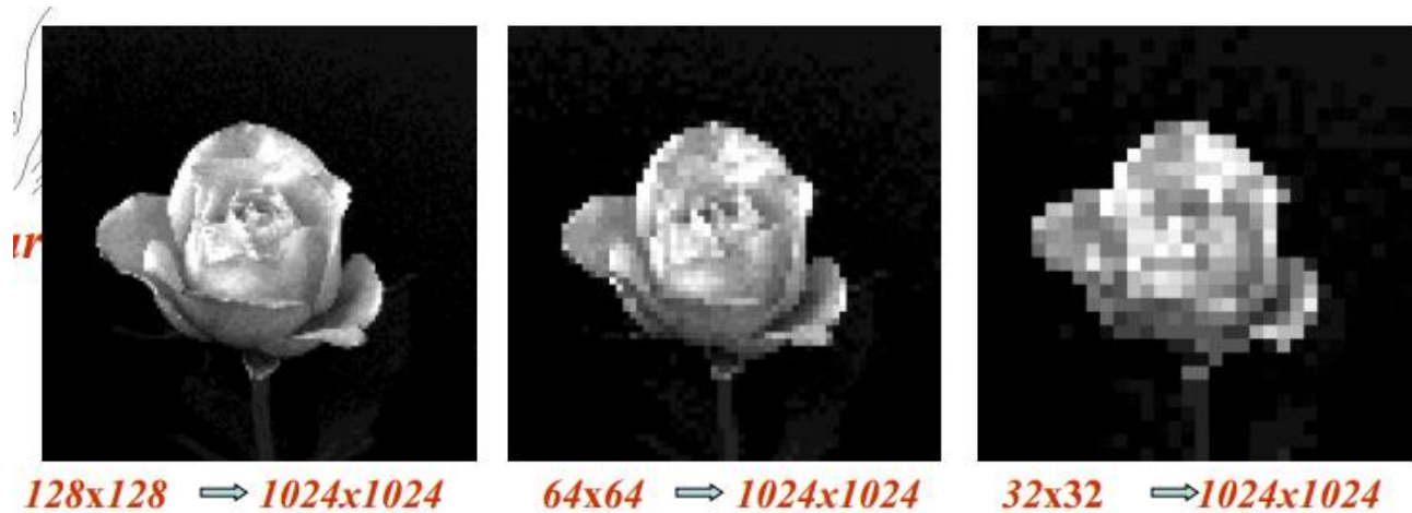
Fig: Images zoomed from 128 x 128, 64 x 64 and 32 x 32 pixels to 1024 x 1024 pixels using nearest neighbor grey-level interpolation.
