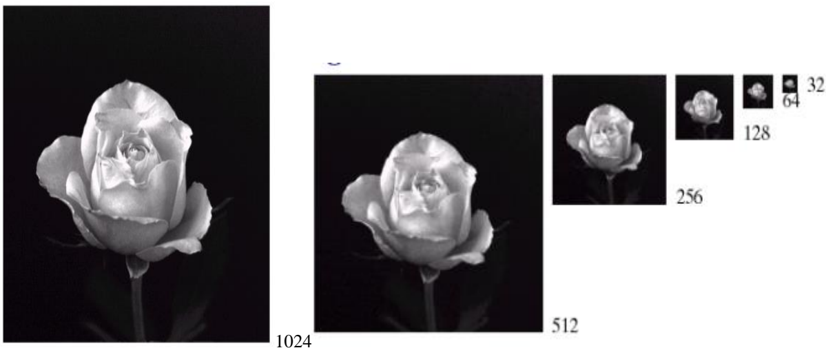
Fig: A 1024 x 2014, 8 bit image subsampled down to size 32 x 32 pixels. The number of allowable kept at 256.
