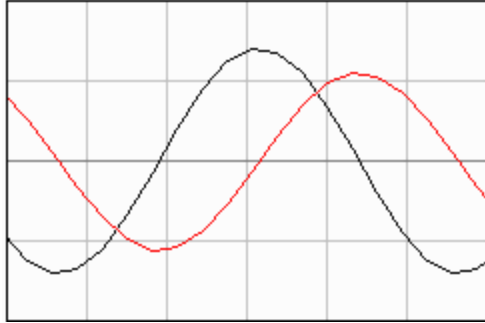
Figure 9.4 - Inductive Phase Shift
