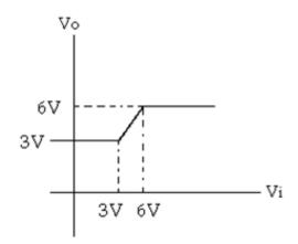
Let  $V_{omax} = 6V$  and  $V_{omin} = 3V$
