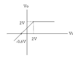
Let the output voltage be clipped at 2V
