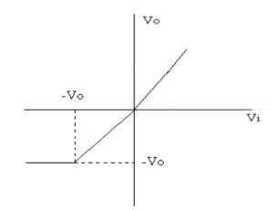
Let the output voltage be clipped at -3V
