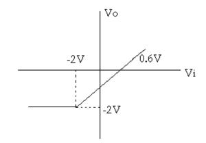
Let the output voltage be clipped at -2V
