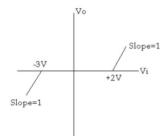
To Clip a sine wave between +2V and -3V level
