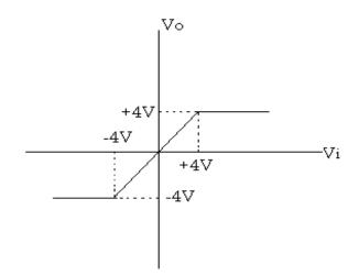
Let  $V_{R1} = V_{R2} = V_R$ ,  $V_{omax} = 4V$
